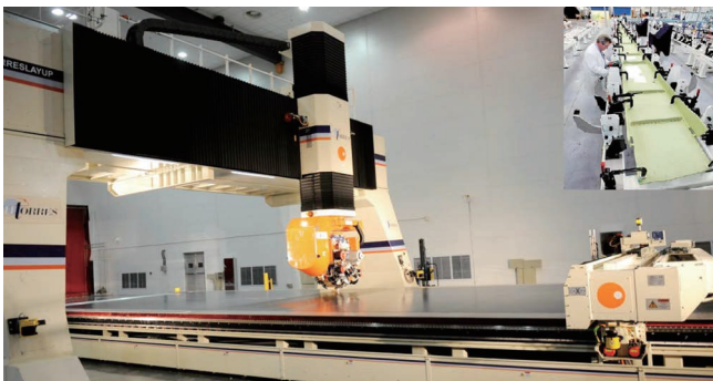
图5 A400M 翼梁采用 ATL 工艺制造 Fig.5 ATL manufacture process of A400M wing spar
