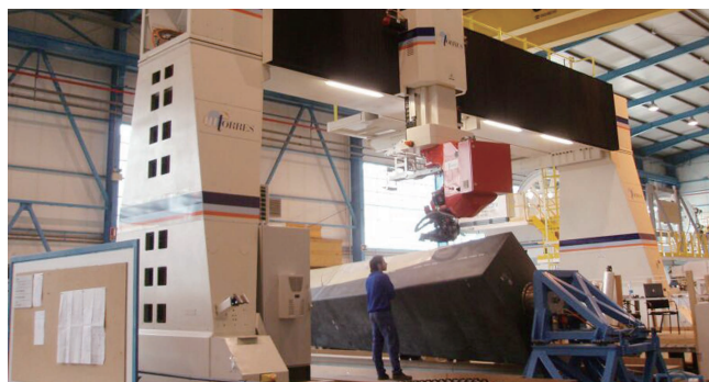
图 9 A350XWB 翼梁 AFP 设备 Fig.9 AFP equipment of A350XWB wing spar
