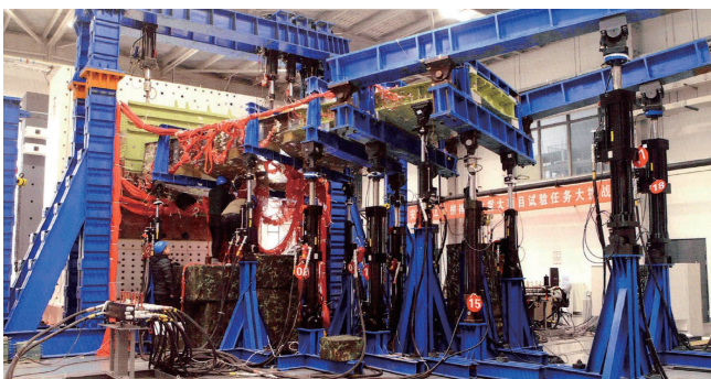
图 11 C919 复合材料机翼研制攻关项目典型盒段静力和损伤容限试验 Fig.11 Static and damage tolerance tests of key projects of C919 composite wing box
