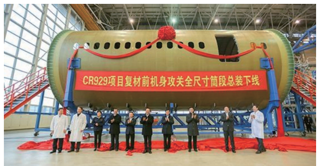
图 12 CR929 飞机前机身攻关复合材料全尺寸筒段 Fig.12 Composite forward fuselage of key projects for CR929 aircraft
